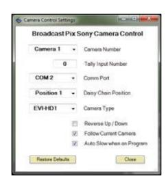
7. Under the **Camera Type** drop down menu, select which style of Sony camera the comport is using, either
